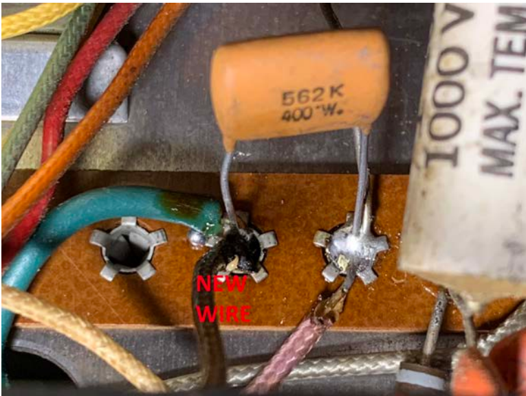
Figure 5b > New wire to GREEN G1 wire term
