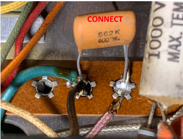
Figure 4 > Connect .047uf, 200v capacitor from violet wire term to GREEN G1 wire term
