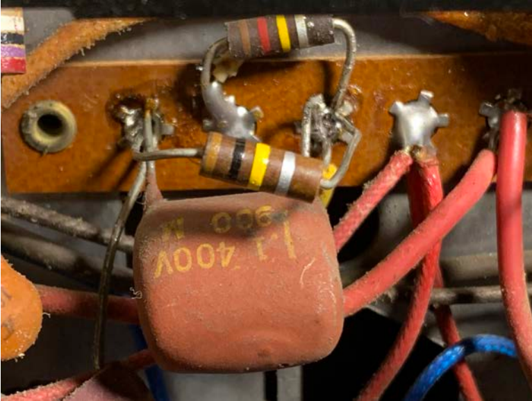
Figure 1 > 100K resistor added in parallel with C29
