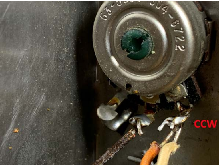
Figure 2 > Yellow wire moved from center term to CCW term
